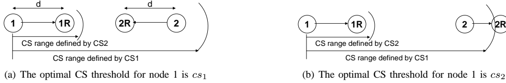
Fig. 8. The optimal CS threshold for node 1 is different for two different network settings.
