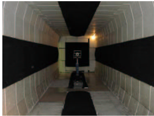
(a) Photo of the inside of an anechoic chamber
