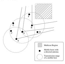
Figure 10. Directed Antenna Utilization for Location-Based Multicast
