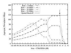
Fig. 3. Aggregate throughput for a circular topology with 32 transmitters
