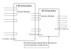
Figure 4. Structure of Scheduling Module
