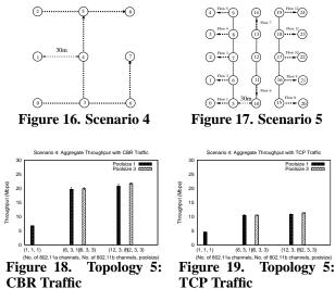
Fig. 17. We vary the number of channels *c*. If *c* channels are in use, the first *c* sources start sending data at t = 40.0s and continue till the end of simulation at t = 50.0s. An ideal omniscient scheduler can assign each flow to a separate channel.
