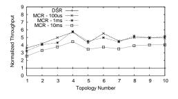
Fig. 10. FTP throughput with varying switching delay
