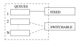
Fig. 2. Illustration of queues associated with N channels and 2 interfaces
