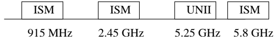
Fig. 4. Chart of commonly used unlicensed spectrum. Spectrum in the 2.4 GHz band is being used by IEEE 802.11b/g devices, and spectrum in the 5 GHz band is being used by IEEE 802.11a devices.
