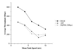
Figure 6: Performance for an FTP source with unlimited data generating traffic across a single TCP connection in a Rayleigh fading channel.
