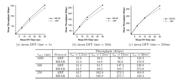
Figure 8: Performance comparison for an ON/OFF Pareto source generating traffic on a single UDP connection in a Rayleigh fading channel. For clarity, the data used for the graphs on top is also shown in the table underneath.
