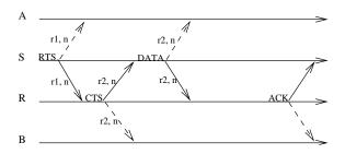
Figure 3: Example packet transfer using the proposed Receiver-Based Autorate (RBAR) protocol.
