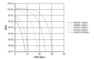
Figure 1: Theoretical bit error rates (BER) as a function of the signal-to-noise ratio (SNR) for several modulation schemes and data rates in an AWGN channel.
