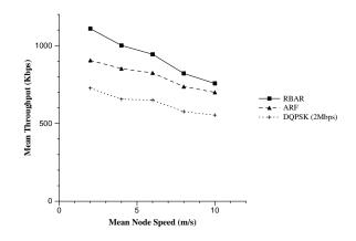
Figure 4: Performance for a CBR source generating traffic on a single UDP connection in a Rayleigh fading channel.
