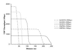
Figure 2: Comparison of throughput versus distance for several modulation schemes. The results were obtained by simulation of a single UDP connection with a CBR source in an AWGN channel with Friis free-space path loss.
