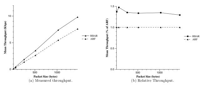
Figure 9: Performance comparison for a Telnet source with interarrival times from the "tcplib" distribution generating traffic on a single TCP-Reno connection in a Rayleigh fading channel.
