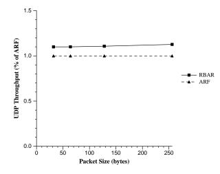
Figure 10: Performance comparison for a CBR source generating traffic on a single UDP connection in a Rayleigh fading channel.
