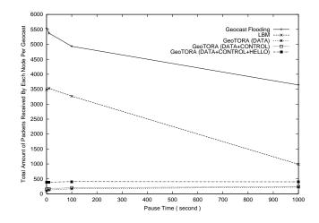
Figure 9: Total Amount of Geocast Packet Delivery (Bytes) versus Pause Time
