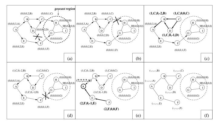
Figure 6: Geocast Route Maintenance in GeoTORA: Three different scenarios of link failure
