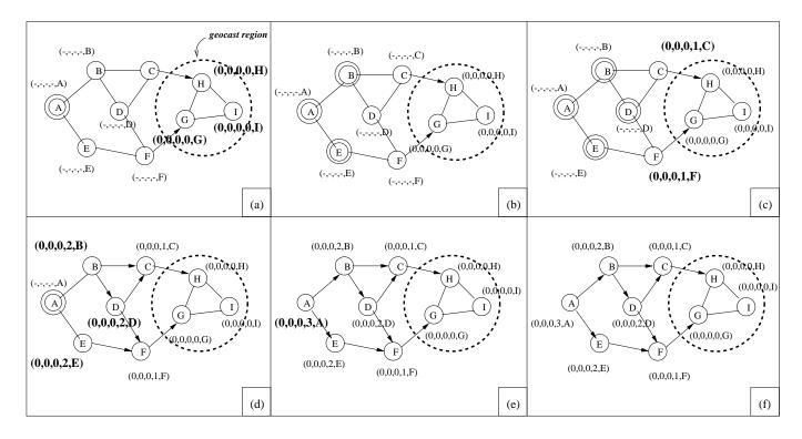
Figure 5: Geocast Route Creation in GeoTORA
