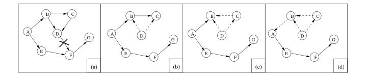
Figure 1: Route Maintenance in TORA: Route maintenance is required due to failure of the link between nodes D and F. In the figure, a link that has been reversed since the initial state is shown as a dashed line.
